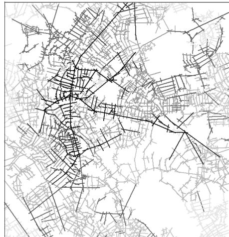
Figure 6 Translation of syntactic properties from a sketch map to an axial map
