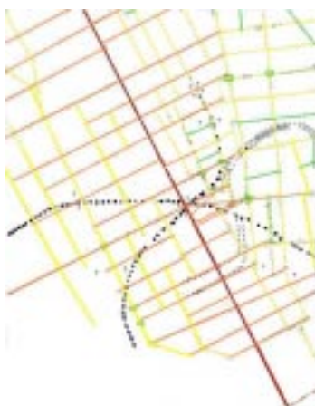
Figure 1: Axial map of Central Stockholm. (The red line marks the assumed integration axis, Drottningatan. The orange lines are one step away the yellow lines are two steps and the green line are three steps away. The black dotted lines mark the Tunnelban and the grey dotted line marks an underground road.)
