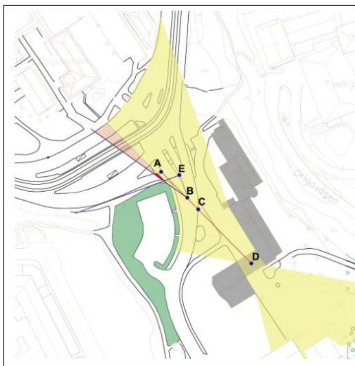
Figure 2: Shaded area is the isovist from point D. Hatched form to the left represents bushes surrounding a parking area. Buildings in black.
