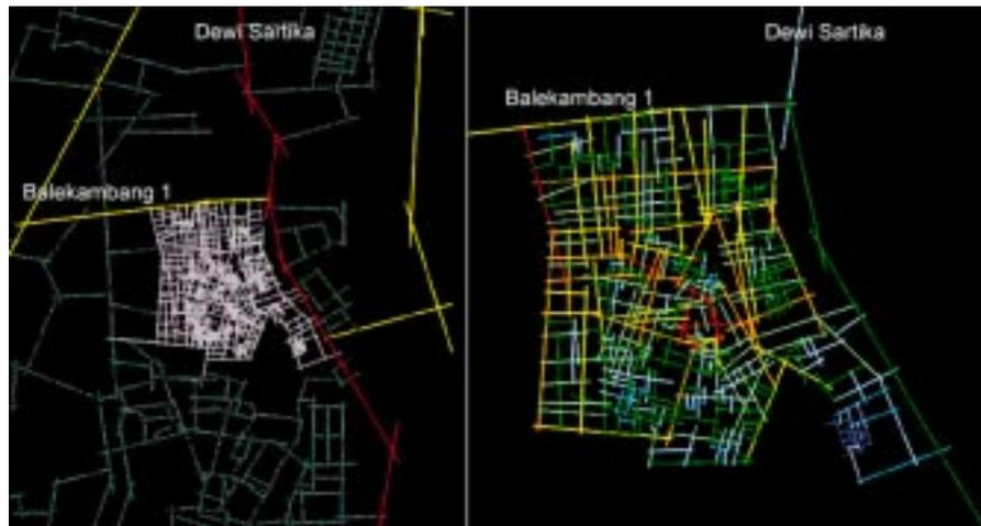
Figure 10: Axial map of Condet, in relation with the surroundings and on its own
