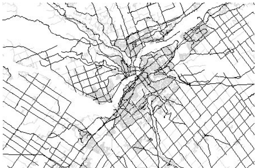
Figure 3: Generalised road network for Ottawa and surrounding area. The retained strokes are shown bold and discarded strokes are shown faint Source: Thomson & Brooks, 2000
