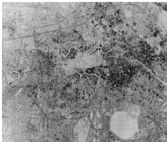
Figure 17. Damaged and Destroyed Buildings in Berlin 1945. Darker buildings were totally destroyed, lighter ones damaged but repairable.
